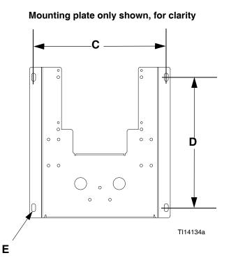
**NOTE:** Height is shown from top of panel to fluid shutoff valves, and does not include the effect of variable fluid integrator heights. Width of panel does not include optional color/catalyst valve stacks.
